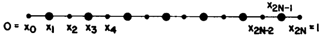
FIG. 1. The unit interval is divided into 2N equally spaced mesh points. The solution is known at x_{2i} but not at x_{2i+1} , i = 0, 1, 2, \dots, N .
